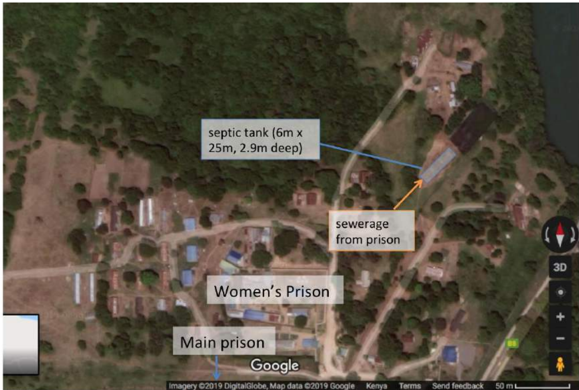
FIGURE 2 – SEPTIC TANK LOCATION
